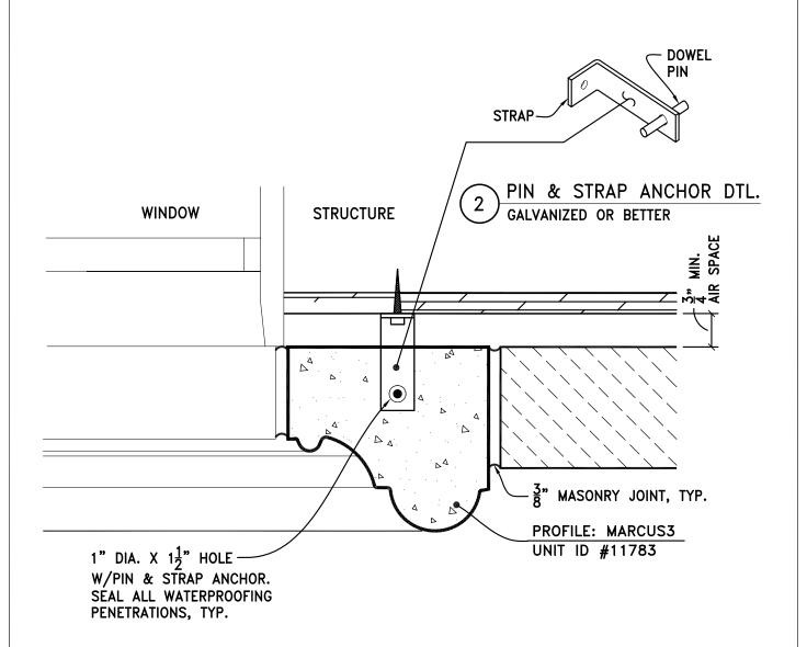
CAST STONE JAMB ATTACHMENT AT MASONRY VENEER WITH PIN & STRAP ANCHOR
